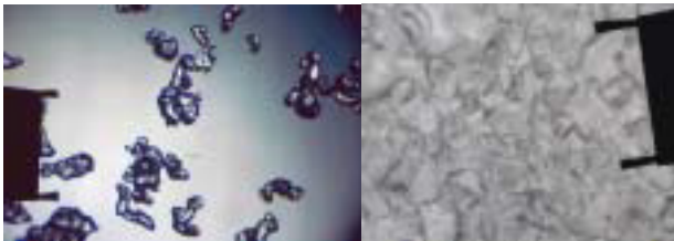
Fig. 1. Original snow crystals and the packed snow surface after sintering. (The grid expresses 1 and 2 mm for the snow crystals and the snow surface, respectively.)
